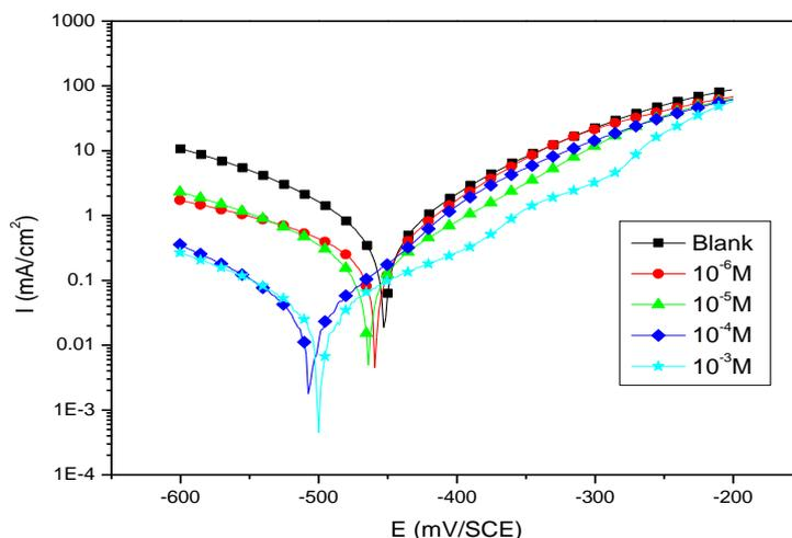
**Figure 1:** Potentiodynamic polarization curves for carbon steel in 1M HCl solution in the presence and absence of different concentrations of MSB at 303 K.
