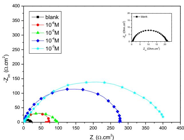
**Figure 2:** Nyquist plots for carbon steel in 1 M HCl solution containing various concentrations of MSB at 303 K.
